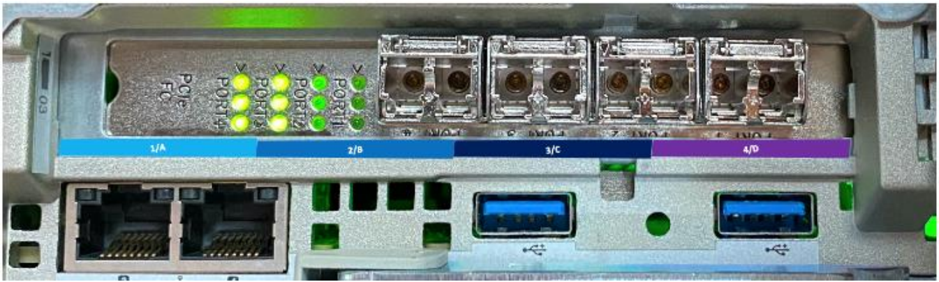
Fibre Channel Interconnect (Controller). The V1000 SE has option of 2 ports
